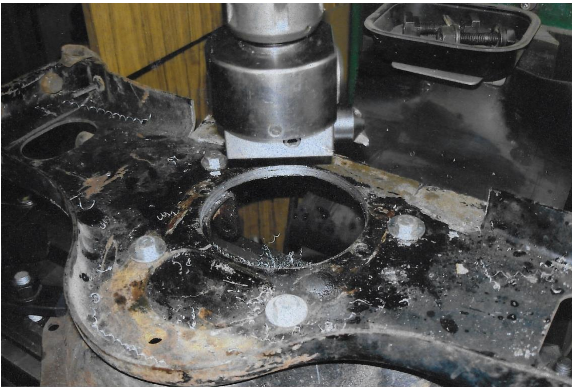
Photo 2: Boring out the X-member
