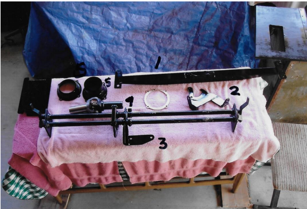
Photo 4: Modified parts including X-member, parking brake mount, cross bar brace, U-joint with S-10 yokes and trunnion ball adapter
