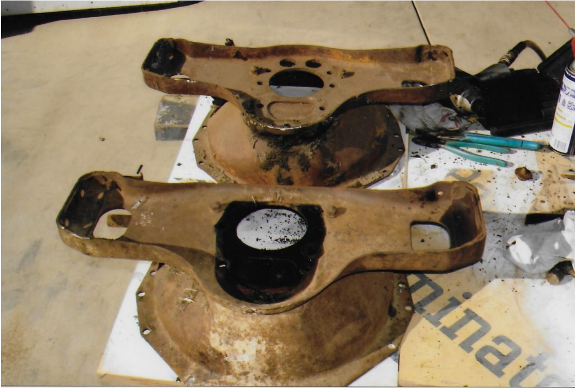
Photo 1: Early Bell housing and X-member (top) and later (28)
